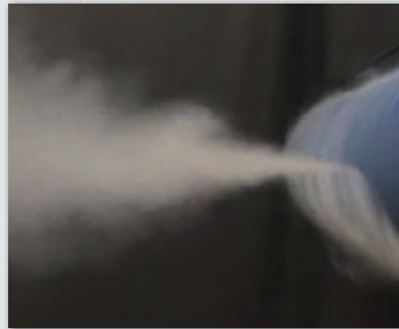
Actual smoke test of air permeable fabric showing thermal barrier and mixing with air dispersion jet
